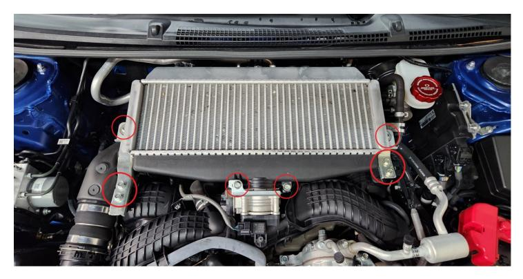
Unclip the charge pipe by pulling this clip up and carefully lifting up on the intercooler and set it aside to expose the PCV hose.
