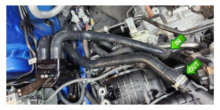
Put the intercooler and charge pipe back in and be sure the charge pipe clip snaps into place. Check all bolts.
