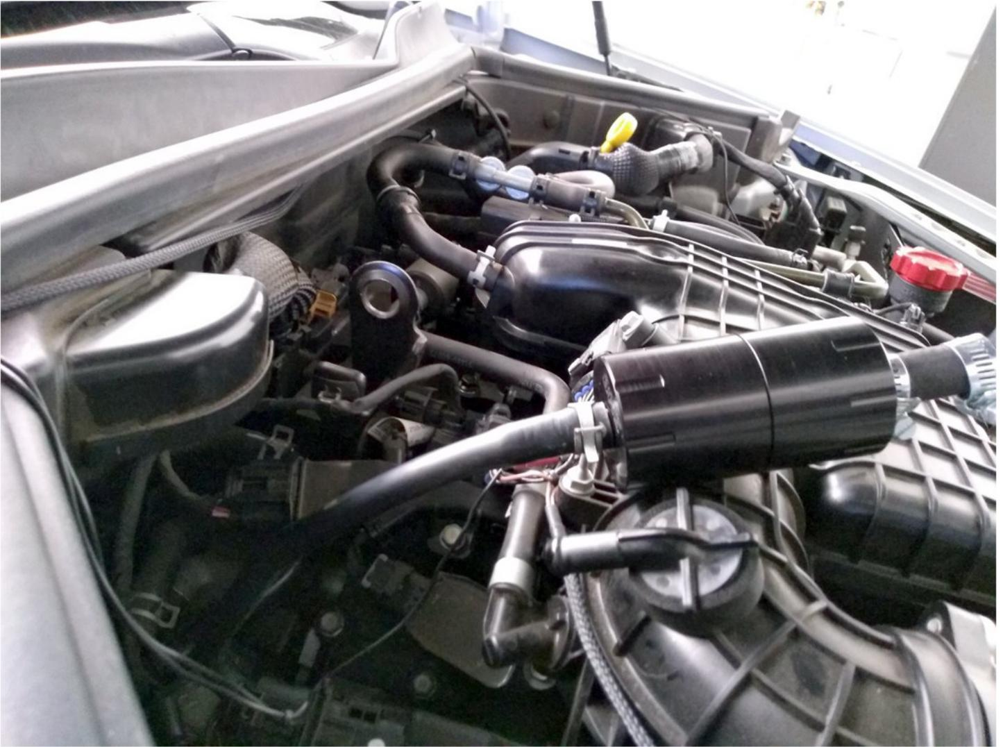
Using the included short hose and worm clamps install the baffle side of the BMS OCC to the factory intake manifold nipple. The OCC does not require a mount and is held in place using the hose connection. Note the short 2" hose provided may be too long for your specific model and can be trimmed as needed to allow a smooth connection to the rear OCC hose.
