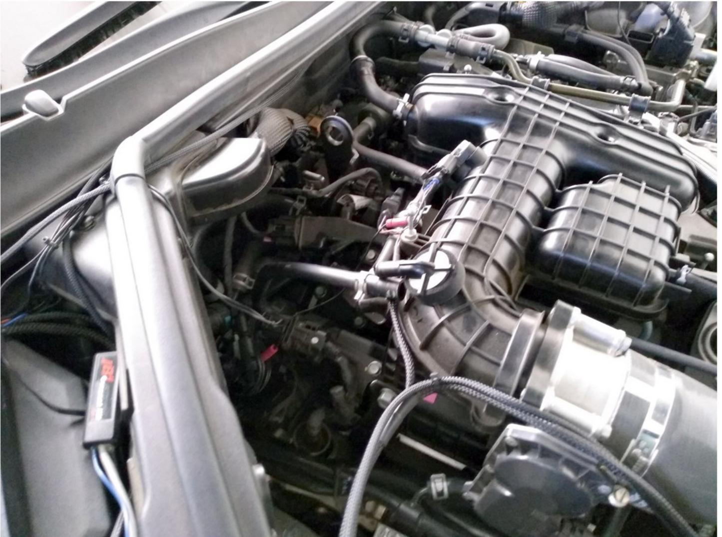
Note the BMS OCC has two sides. The baffled side that also has machined screws in cap should face the intake manifold.
