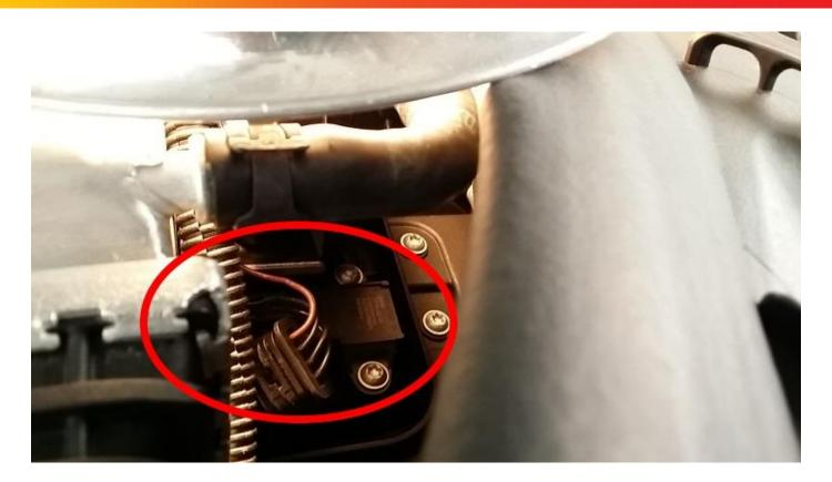
For the Stage1 installation these are the only harness wires used. The rest can be tucked out of the way.
