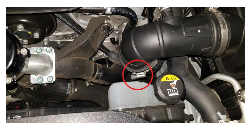
Loosen the hose clamp that holds both the left and right intake inlets with either a flat head screwdriver or a 10mm socket. Left shown above and right shown below. Leave the hose clamp in place after loosening.
