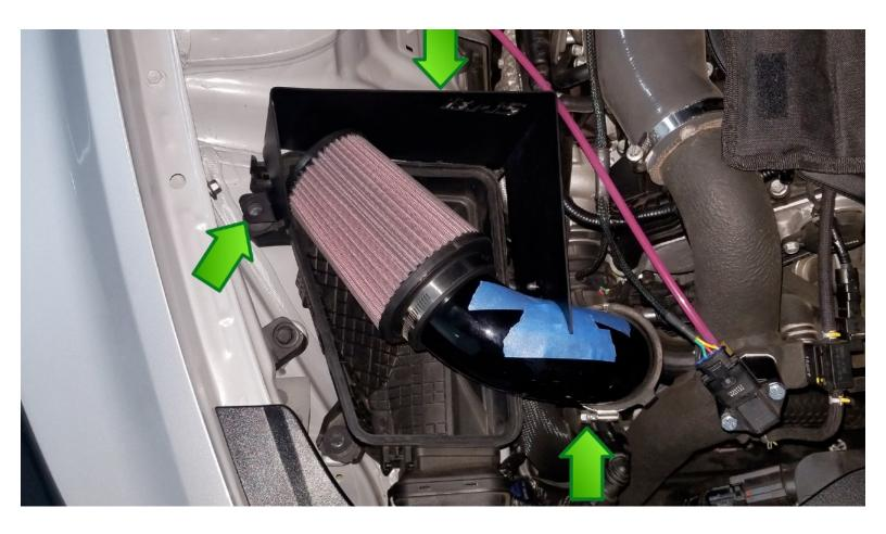
Place the intake and heat shields on top of the factory air box bottom. Make sure the metal tubes are all the way in as far as they can go in the factory inlets and tighten the hose clamps on both sides of the car. Next bolt the heat shield down with the 10mm bolts you removed. Do this on both sides.
