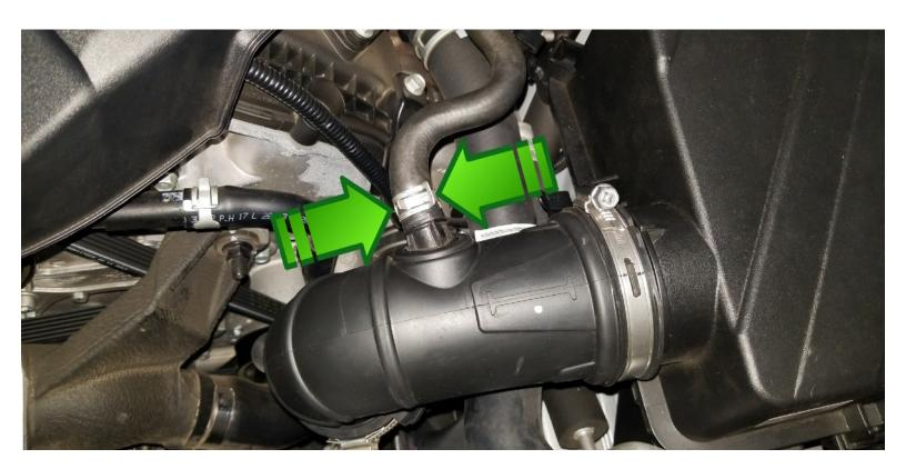
Now on the left side of the motor remove the vacuum hose by pinching the metal tabs with pliers and pulling the hose straight off of the nipple.
