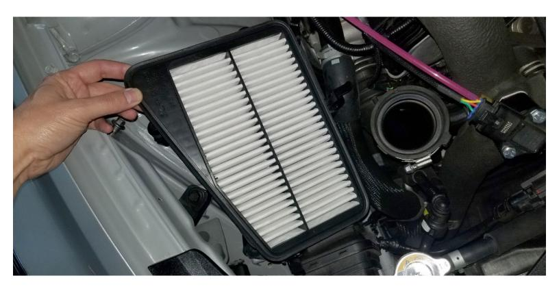
The metal airbox clips still attached to the lower half of the airbox need to be removed. They can be removed by tilting them all the way inward and pushing forcefully down to unclip. Keep these with your factory parts.
