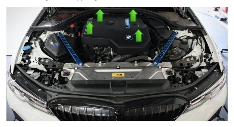
Attach the supplied bracket to front two holes in the lid of the BMS oil catch can. None of the 4 screw holes should be visible with the bracket in place.
