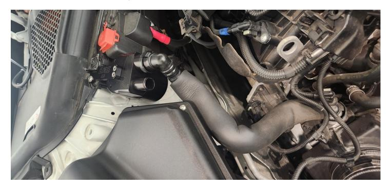
Put the included silicone hose on the IN fitting on the can and the other end over the PCV outlet on the engine. Clams are not required. The PCV system is low pressure.
