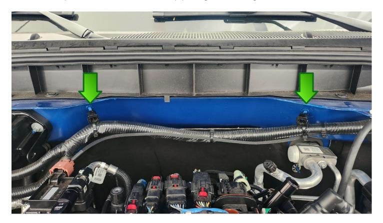
Next place the supplied custom bracket on them and secure it with the supplied 10mm flanged nuts. Then place the wire loom back in place.
