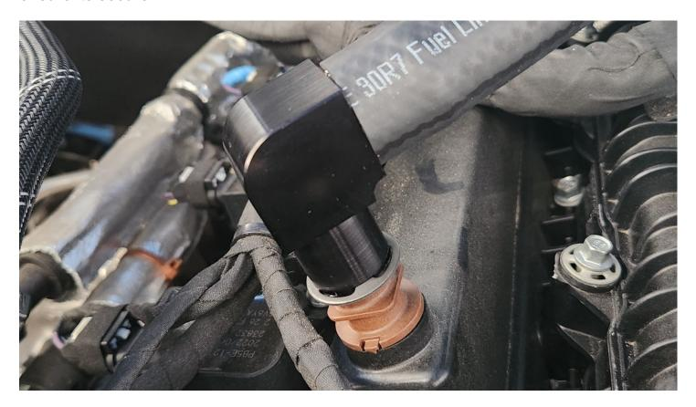
Install complete. Simply unscrew the base every 3-6 months to empty or use the 1/8th NPT drain plug.
