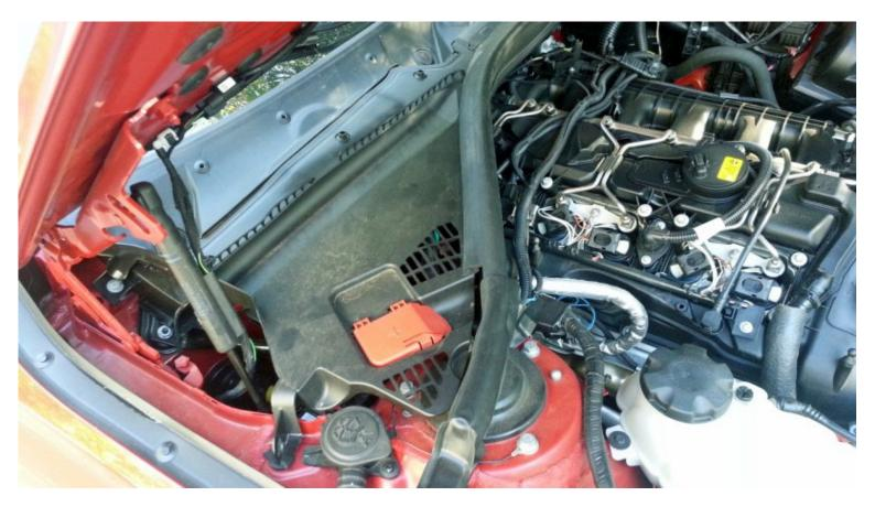
7) Reinstall the engine cover by pressing it back in place on top of the engine.
