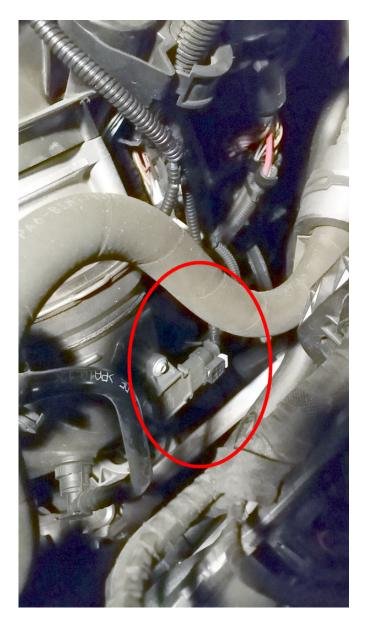
4) The MAP sensor is located on the top of the engine towards the back under engine foam. It is visually identical to the TMAP sensor. Disconnect the MAP sensor plug and plug it in to the JB female brown connection. Plug the male brown connection in to the MAP sensor completing the loop.
