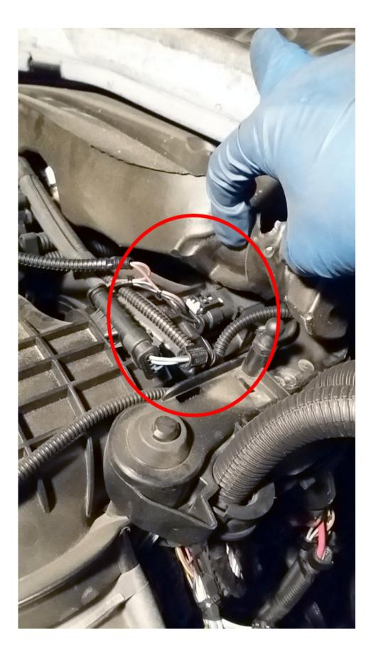
5) The Stage 1 control box should be placed under the passenger side plastic cover as shown. For long term installations we suggest using a zip-tie to secure it to the strut brace. For short term installations it can simply sit in place. Take care to avoid accidentally contacting the 12v battery jumper nut while working in this area.
