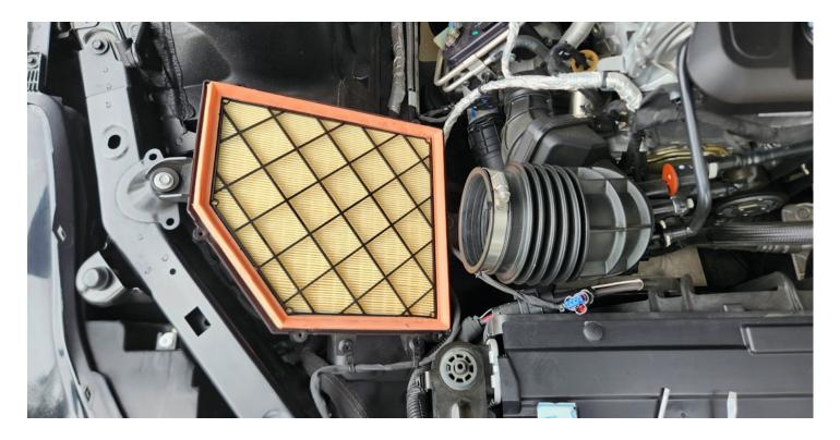
Assemble the BMS intake and filter. Be sure to tighten all of the bracket bolts. They can be used for slight adjustment if needed. Install the MAF sensor with the supplied allen bolts. Tighten the filter clamp but don't over-tighten.
