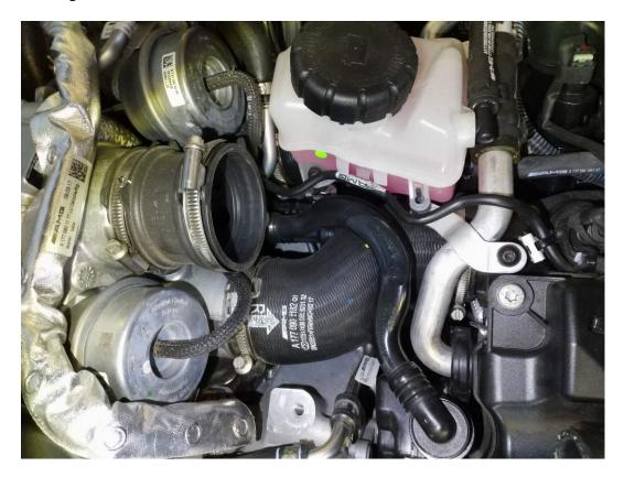
Loosen the clamps holding the rubber coupler in place. Using a screwdriver or other pry tool, release and remove the coupler. Repeat for the driver's side coupler.
