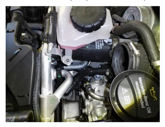
Install the silicone couplers on each side. Suggested hardware orientation and line routing shown.
