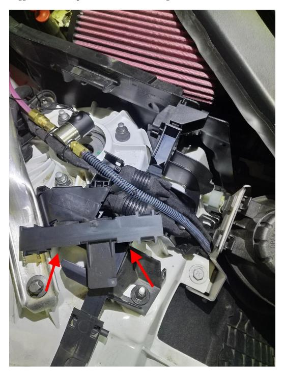
Make sure to replace the plastic cover shown after routing the line. Extend one solenoid wire and connect at the ground location used for the meth pump. The other will be connected in a later step. Teflon paste should be used a the threaded connections into the solenoid. Note the direction of the arrow on the solenoid noting flow. The filter should be placed on the inlet side of the solenoid, again noting the flow direction arrow.
