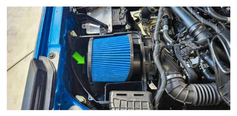
The BMS filter should sit straight up and down in the airbox bottom.
