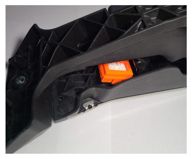
When the unit is properly aligned, the factory detent button will be in the center of the window and the unit will be aligned to the pedal surface.
