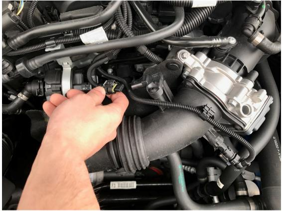
TMAP Sensor for X1 and MINI Models. Note this specific JB+ will have 4 wires:
