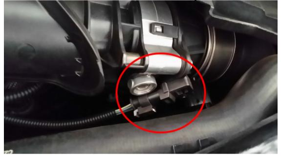
3. Unplug the factory plug by pressing down the tab or by using a small screwdriver on the back side to lift up the clip from the back and sliding the connector off the sensor. Plug the factory sensor wire in to the JB+ and plug the JB+ in to the sensor.
