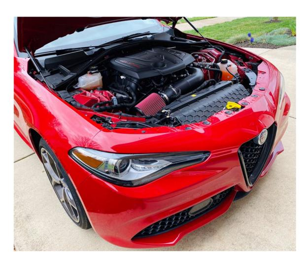
Remove the factory airbox top and MAF housing by unscrewing the accordion tube, unplugging the MAF sensor, and unscrewing the perimeter bolts securing the airbox top to the airbox bottom.
