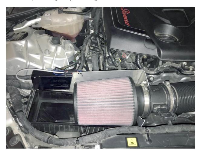
Line up the heat shield with the factory airbox and screw down using the factory screws to secure the new assembly to the airbox bottom.
