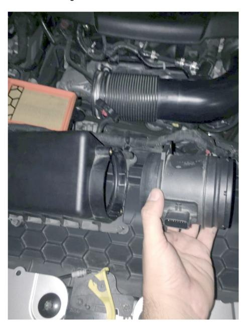
Push the BMS intake filter over the factory MAF housing and secure it using the included clamp. Align the BMS intake heat shield with the factory MAF housing and secure it using the included bolts/nuts.
