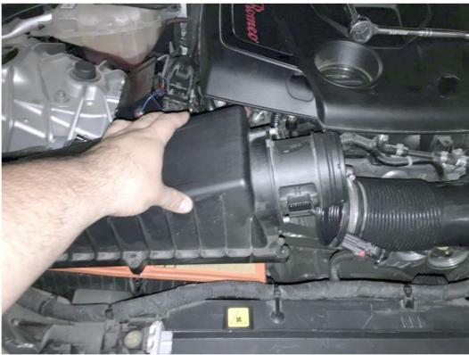
Disconnect the MAF housing from the airbox top by removing the screws attaching it. We'll be reusing this with the BMS intake.
