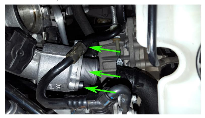
If your having trouble removing the factory turbo muffler from the engine compartment you may need to remove the plastic turbo inlet pipe. Loosen the torx bolt circled below. Then turn the turbo inlet towards the back of the car and pull it out to the right.
