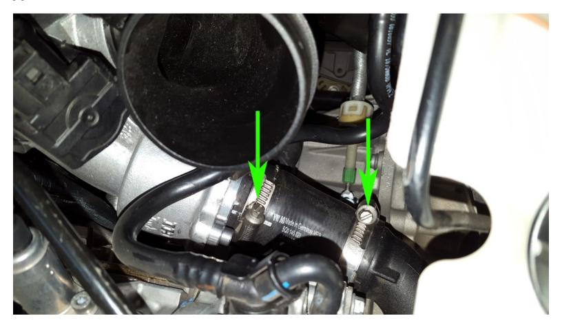
Remove the 3 allen bolts from the factory turbo muffler and carefully remove it. Be careful with the thin rubber gasket inside. Be sure to return it to its groove if it falls out.
