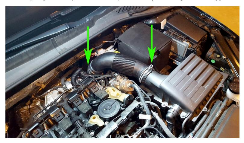
Loosen the hose clamps on the hose attached to the factory turbo muffler and remove the hose. You can pull the plastic pipe a little to aid in removal of the rubber hose.
