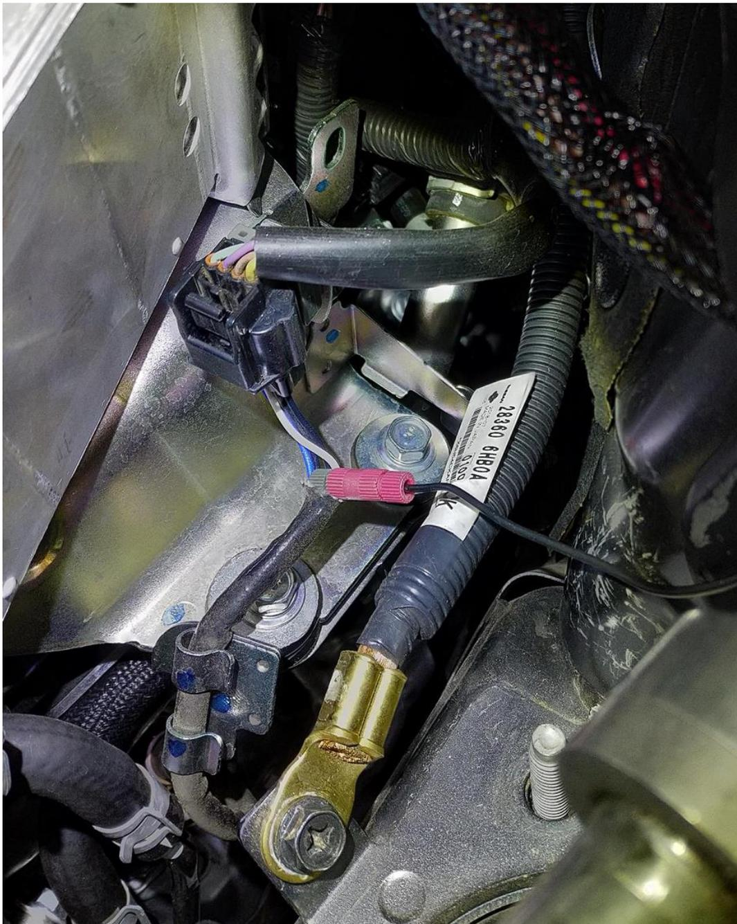
The passenger side fuel wire connection is in a mirror location on the opposite side of the engine compartment. Attach the Posi-tap connection to the white wire in the factory wire bundle.
