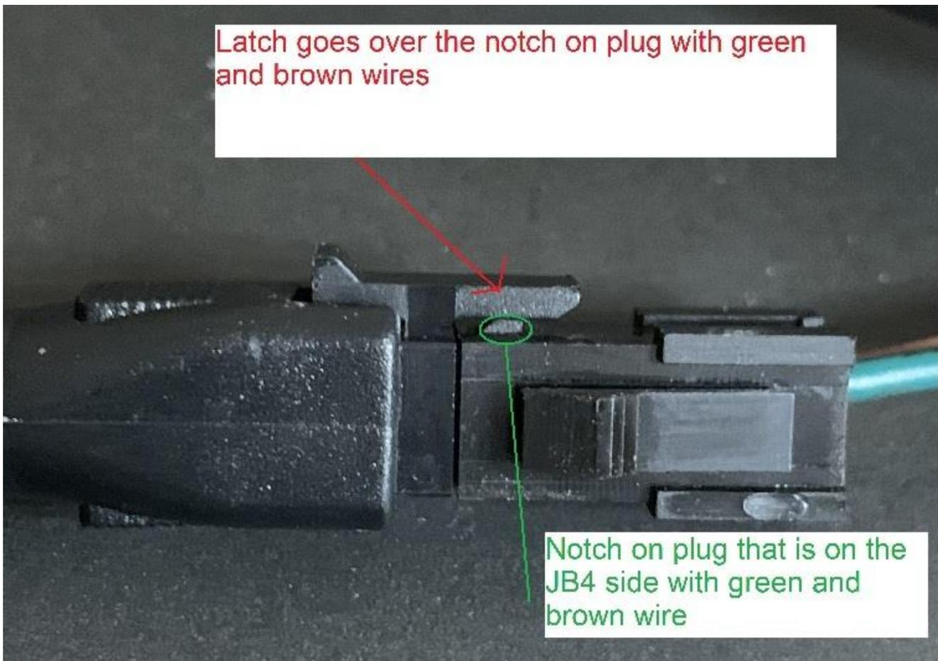
Notch on plug that is on the JB4 side with green and brown wire
