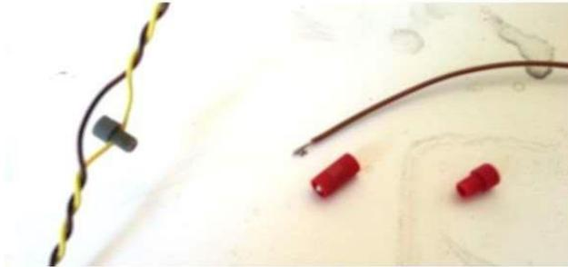
Slide wire to be connected through connector as shown and poke stripped wire in to base. As you tighten base ensure wire remains inserted and that the wire makes a solid connection.
