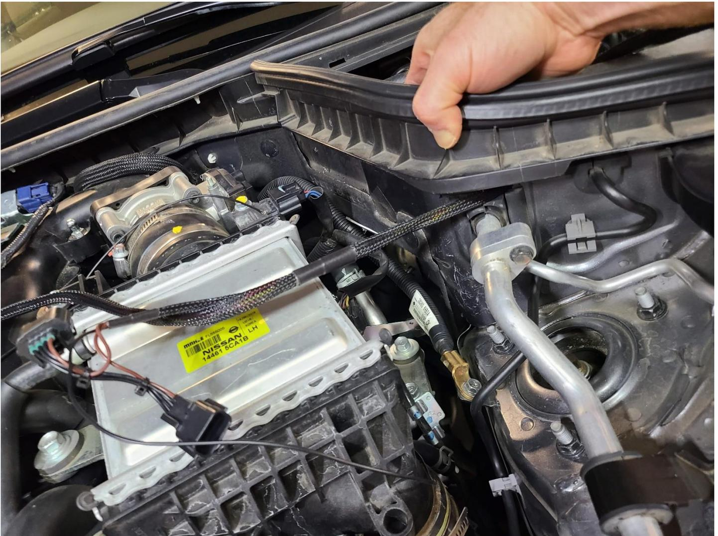
The JB4 or Stage1 connects to two MAP connections under the hood. The rainbow connection goes to the passenger side sensor while the brown wire connection goes to the driver's side sensor.
