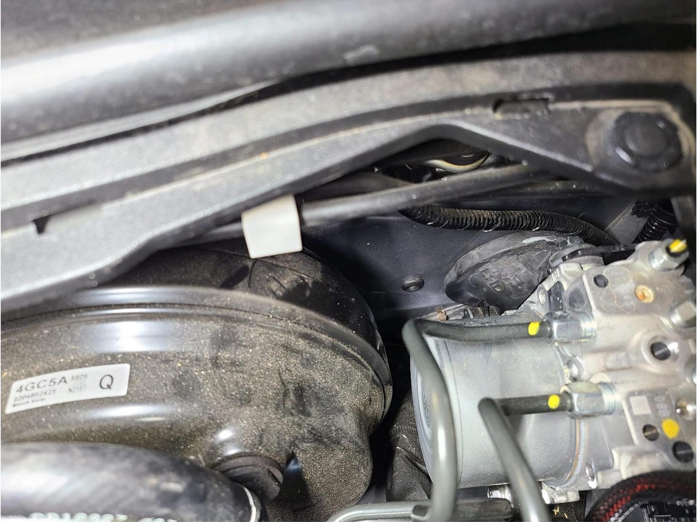
Under the dashboard to the left of the parking brake pedal, locate the wire harness passing through the grommet.
