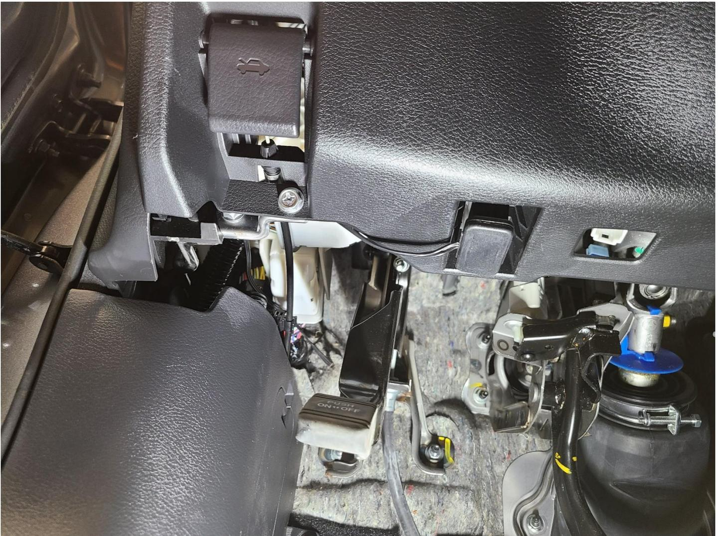
Return to the area near the brake booster to find the end of the OBDII cable that you passed through in a previous step. Pull gently on the end of the wire and bring the end toward the JB4's control box. Pull the bulk of the wire through into the corner compartment, leaving just enough slack for the OBDII cable to reach the OBDII port. The wire should not be under tension so make sure there is enough slack in the footwell.
