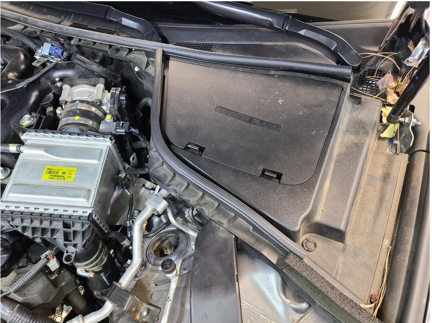
Place the JB4 or Stage1 control box as shown near the brake booster.
