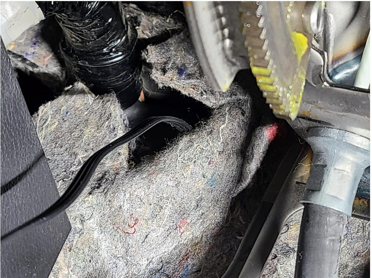
Attach the large end of the OBDII cable to the OBDII port as shown.
