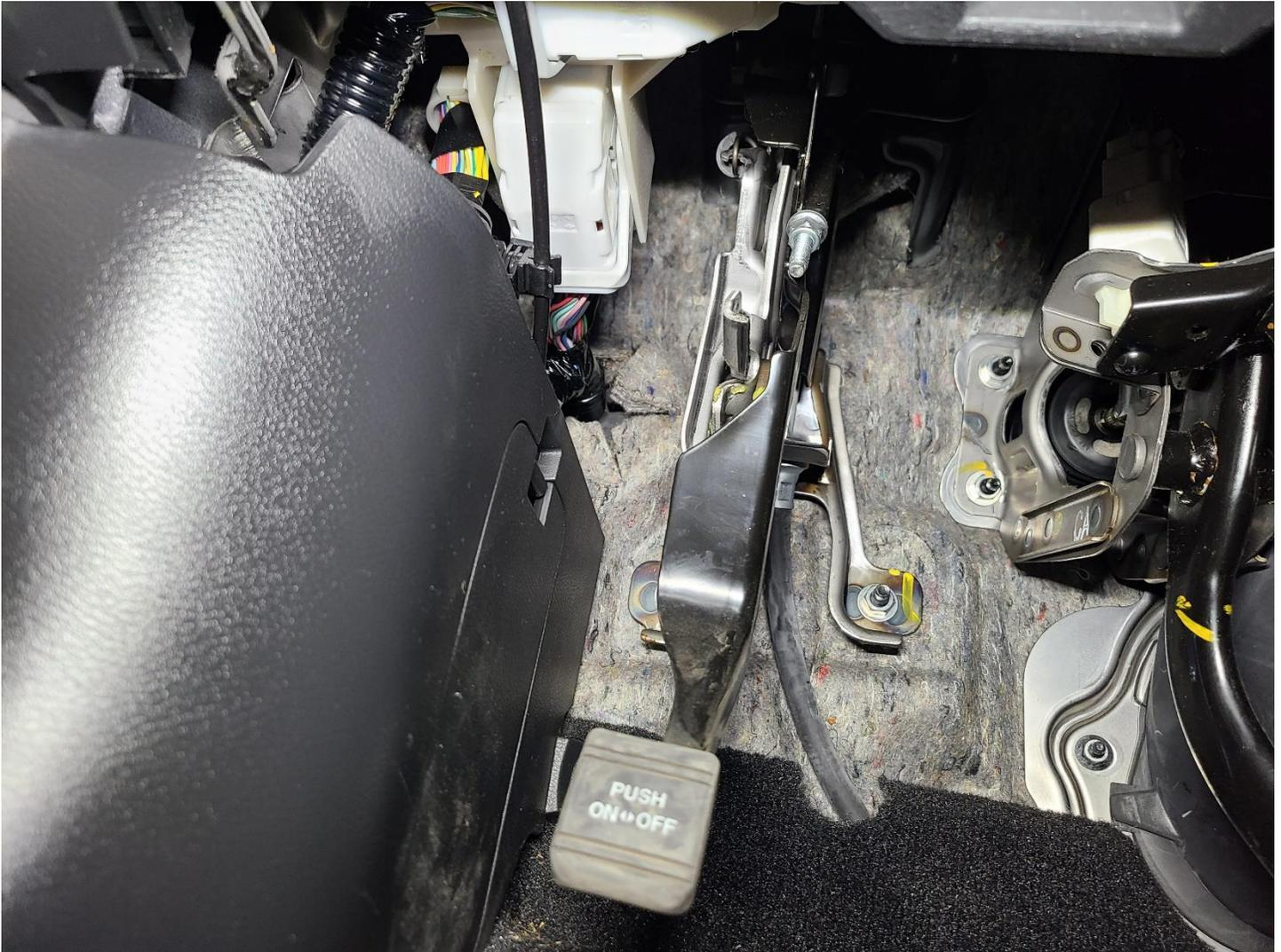
You can push on the grommet with a screwdriver or your fingers toward the engine compartment. Then pass the small end of the OBDII cable next to the grommet.
