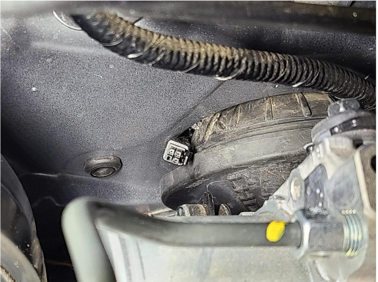
You can now replace the grommet by pressing from the corner compartment. Note that the arrow must line up with the dot on the firewall for the grommet to fully seat and seal over the OBDII cable.
