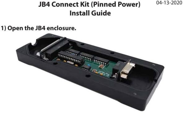
2) Install the DB9 connector and ensure both screws are secure.
