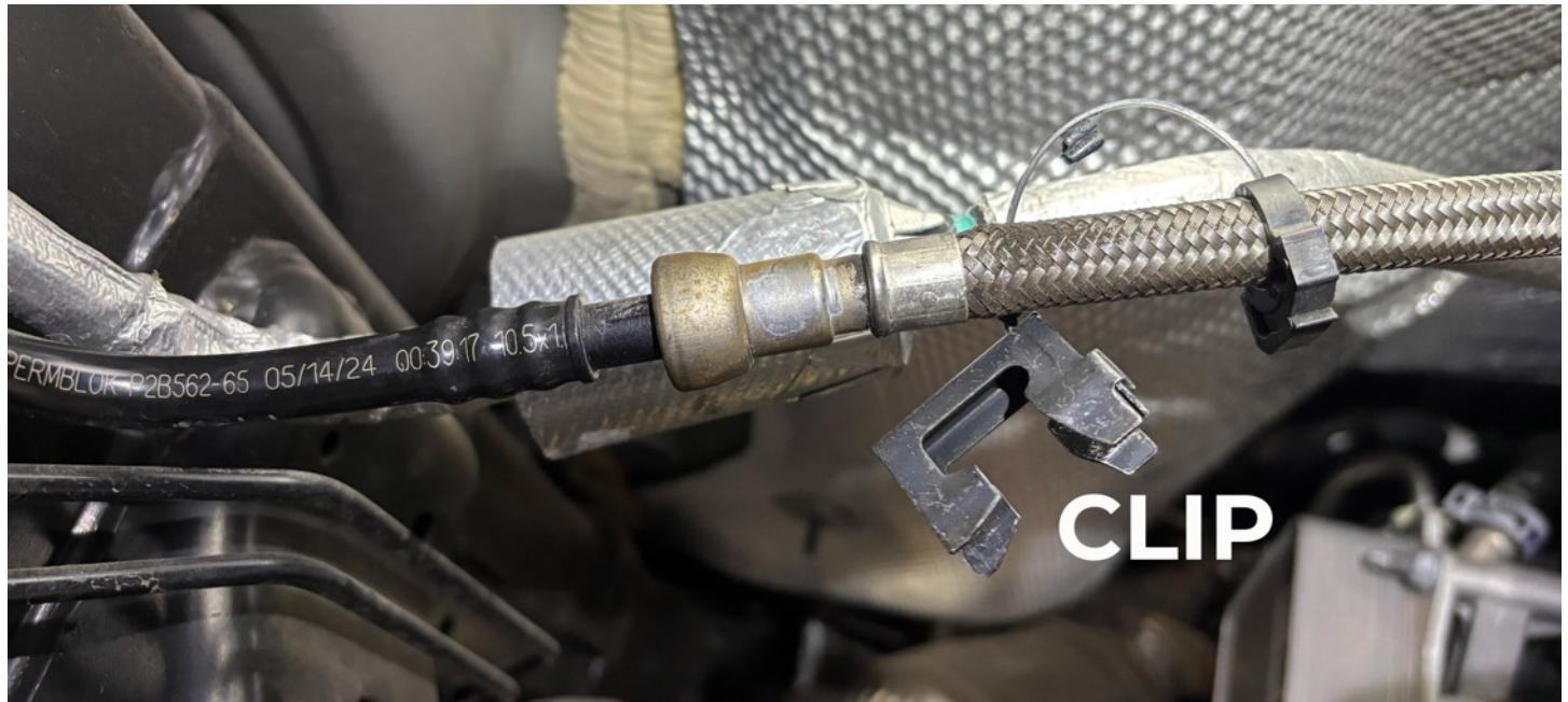
Press the included fuel line unlock tool into the metal fuel line to release it.
