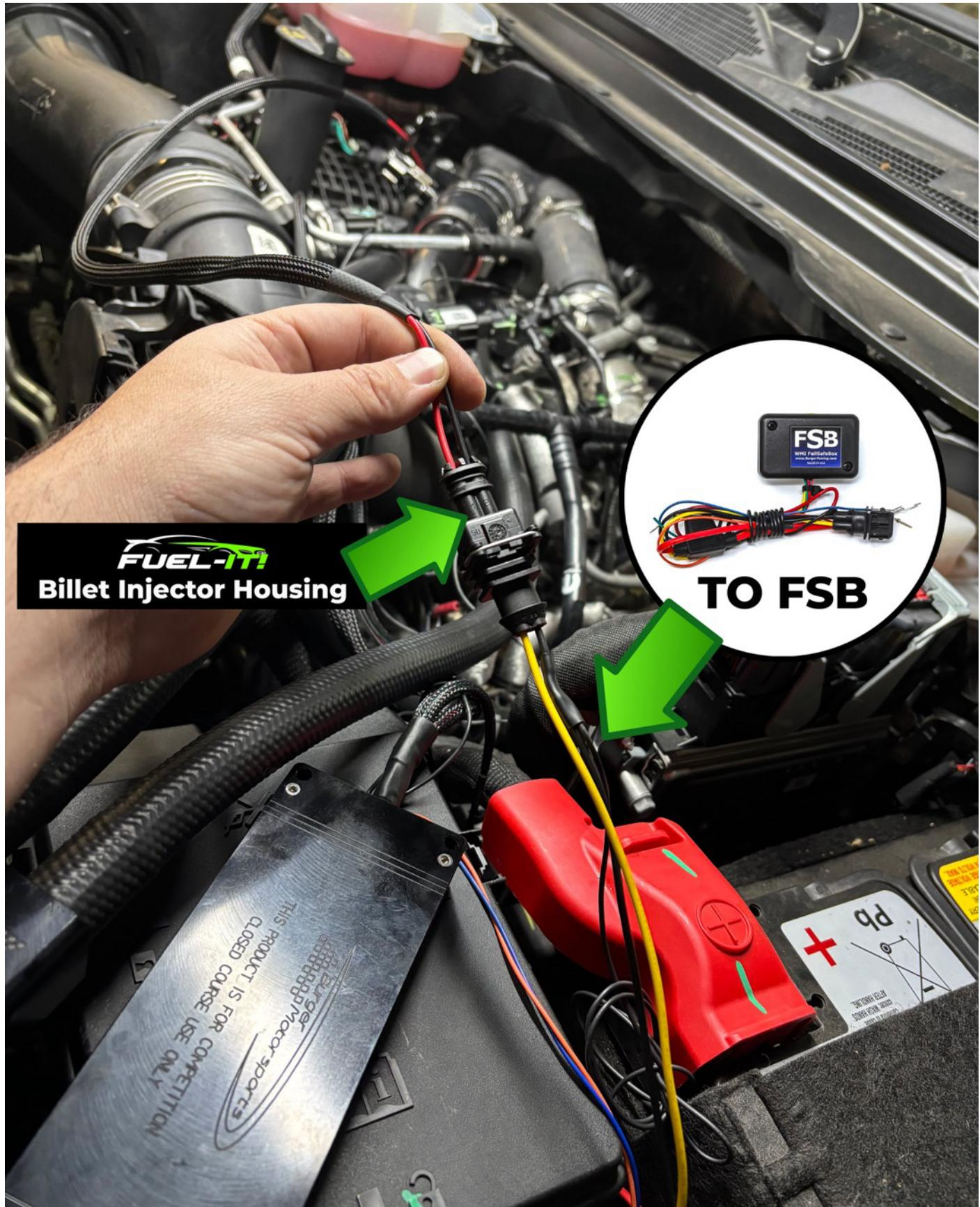
The FSB has two pins that plug in to the JB4 connector. Open the JB4 control box and route the blue and orange wires **through the JB4 grommet**. Insert the orange wire in to spot #3, and the blue wire in to spot #16.
