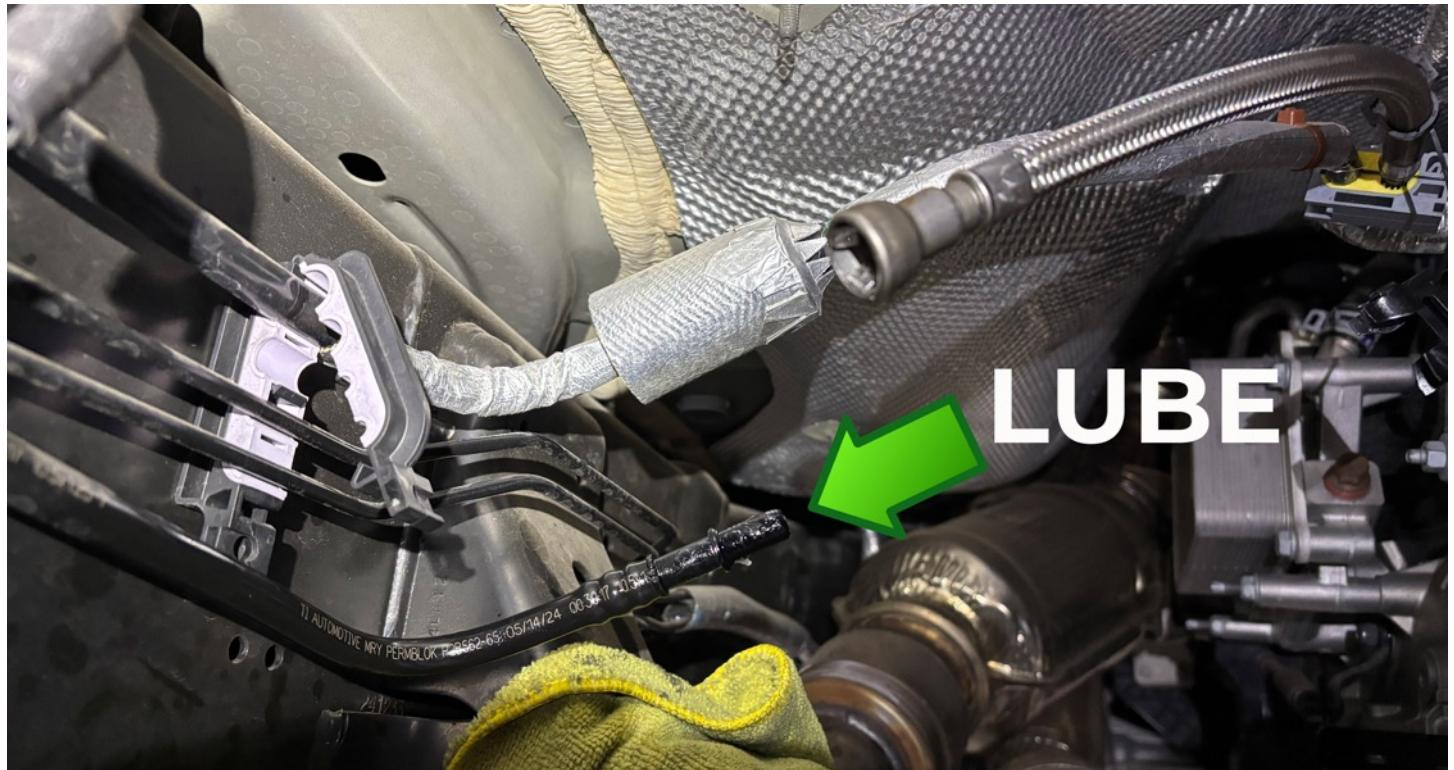
Now put the included fuel line adapter in-between the factory braided fuel line and plastic fuel line. Be sure to lube both ends of the line before assembly.
