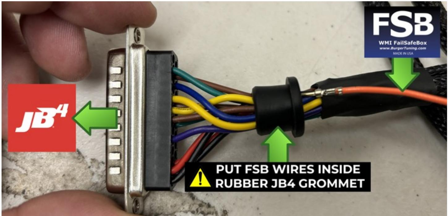
Note pins on the JB4 connector are labeled on both sides. (top and bottom)
