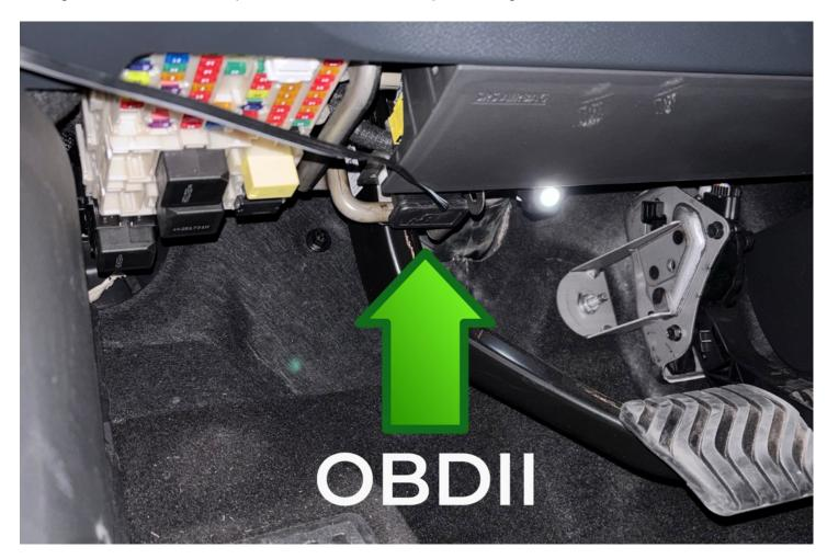
Finally plug OBDII into JB4 harness, note correct clip over notch orientation. If no data appears in JB4 app once connected an issue with the OBDII connection is usually the culprit.
