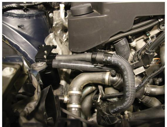
Now just place the intake box back on. Place the thin hose back in the brackets on the top rear of the intake box. Connect the hose clamp area and the MAF sensor wires. Make sure it clicks in. Make sure the intake box is secure at all 3 contact points and you are done. Enjoy an oil free intake system and prolonged engine life.
