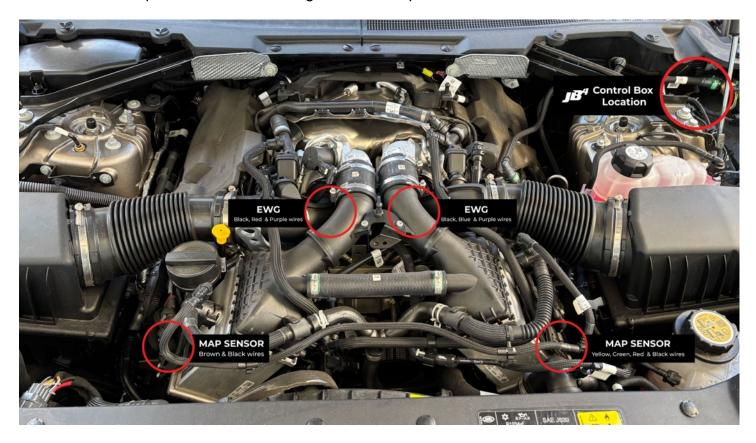
First unplug the factory MAP connector on the left side of the left intercooler. It's the 3rd plug down.
