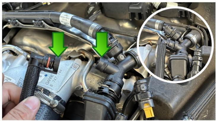
Now remove the right side (facing the engine) turbo inlet by unplugging the temperature sensor and pulling up on the large circlip on the turbo inlet and pull it towards the front of the vehicle to remove.
