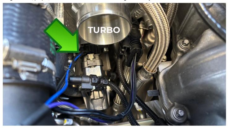
Unplug the left (facing the engine) EWG connector with the red, blue, purple, and black wires. Plug the factory connector in the other end.
