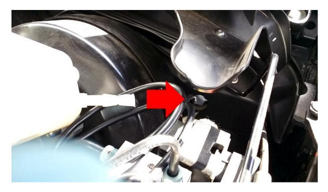
Note those with a manual transmission have the clutch line run through this same hole. You'll need use a coat hanger to pull CANbus wire around the grommet. Alternatively you can use cut a small slice in the grommet to facilitate feeding the CANbus wire through.
