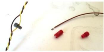
Slide wire to be connected through connector as shown and poke stripped wire in to base. As you tighten base ensure wire remains inserted and that the wire makes a solid connection.
