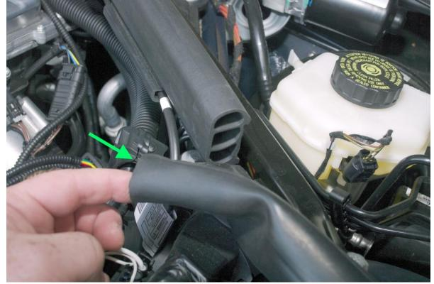
Now run the JB wire harness between the split in the weather seal and replace the weather seal as shown. The portion of the wire harness with the AMP cover on the connector should now be near the brake booster.
