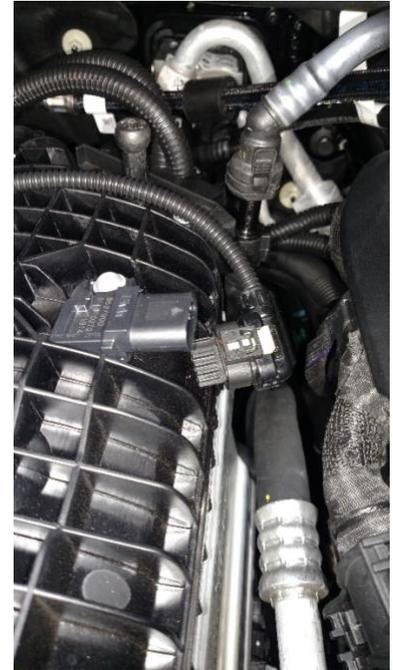
Connect the red, green, black, and yellow JB4 patch wire connectors to the stock manifold sensor and stock connector.
