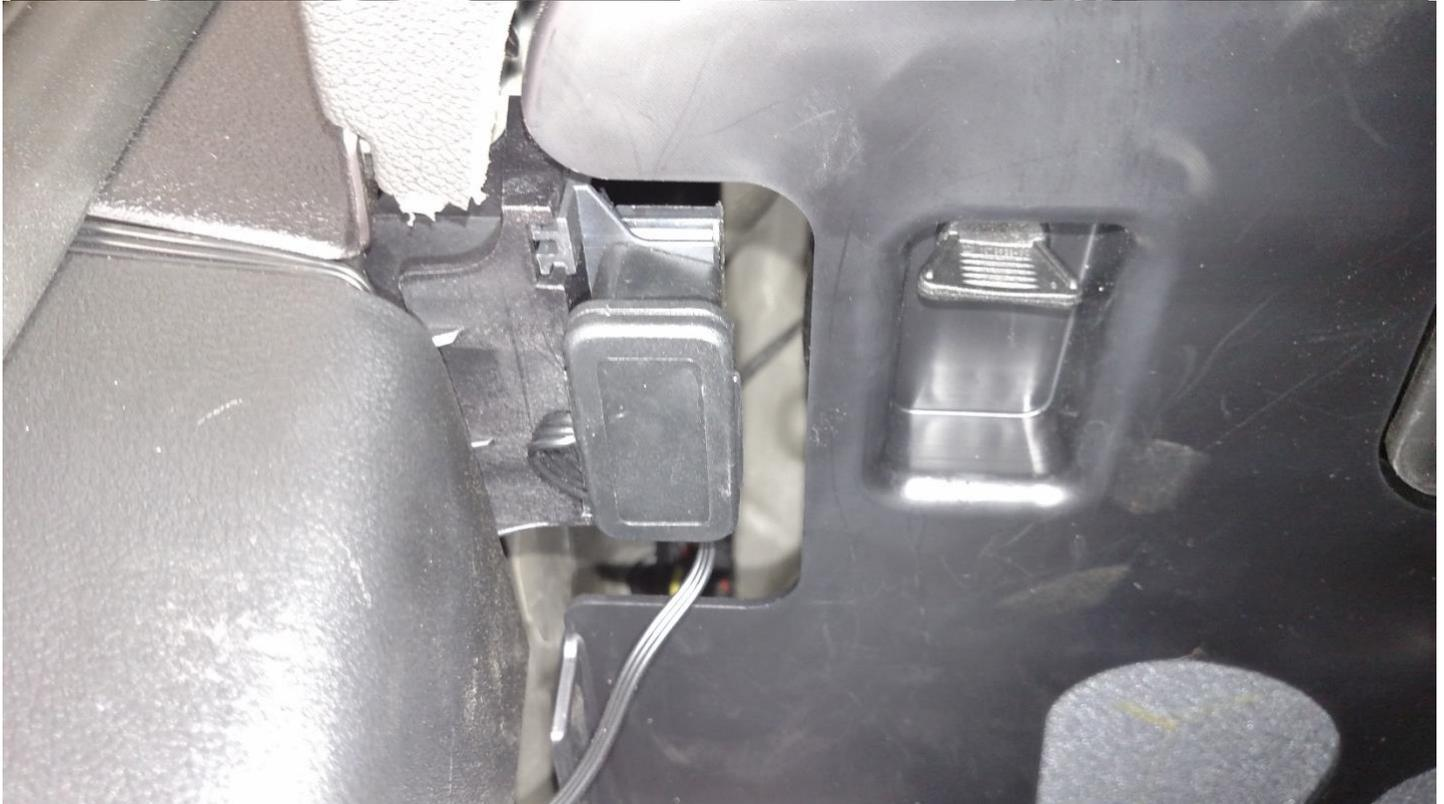
OBDII Option 2: Use a knife to pierce this existing hole. Route the JB4 OBDII cable to the driver's side under the dash through the hole in the firewall and plug in to the OBDII port under the dash near the driver's side door. Top pic: X3M/X4M Bottom Pic: M3/M4
