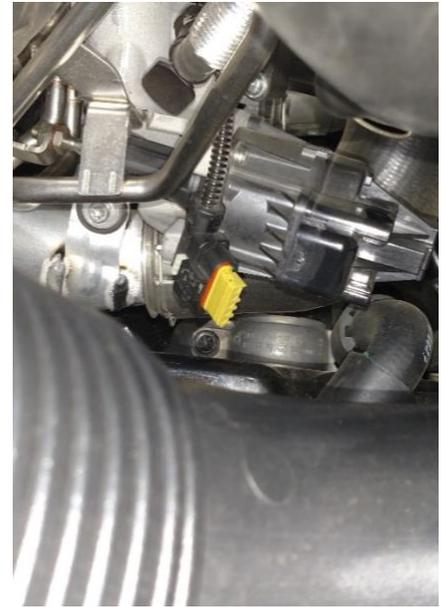
Plug the JB4 harness in to the wastegate controller and plug the stock connector in to the JB4 harness for both turbos. Note: There is no particular order.
