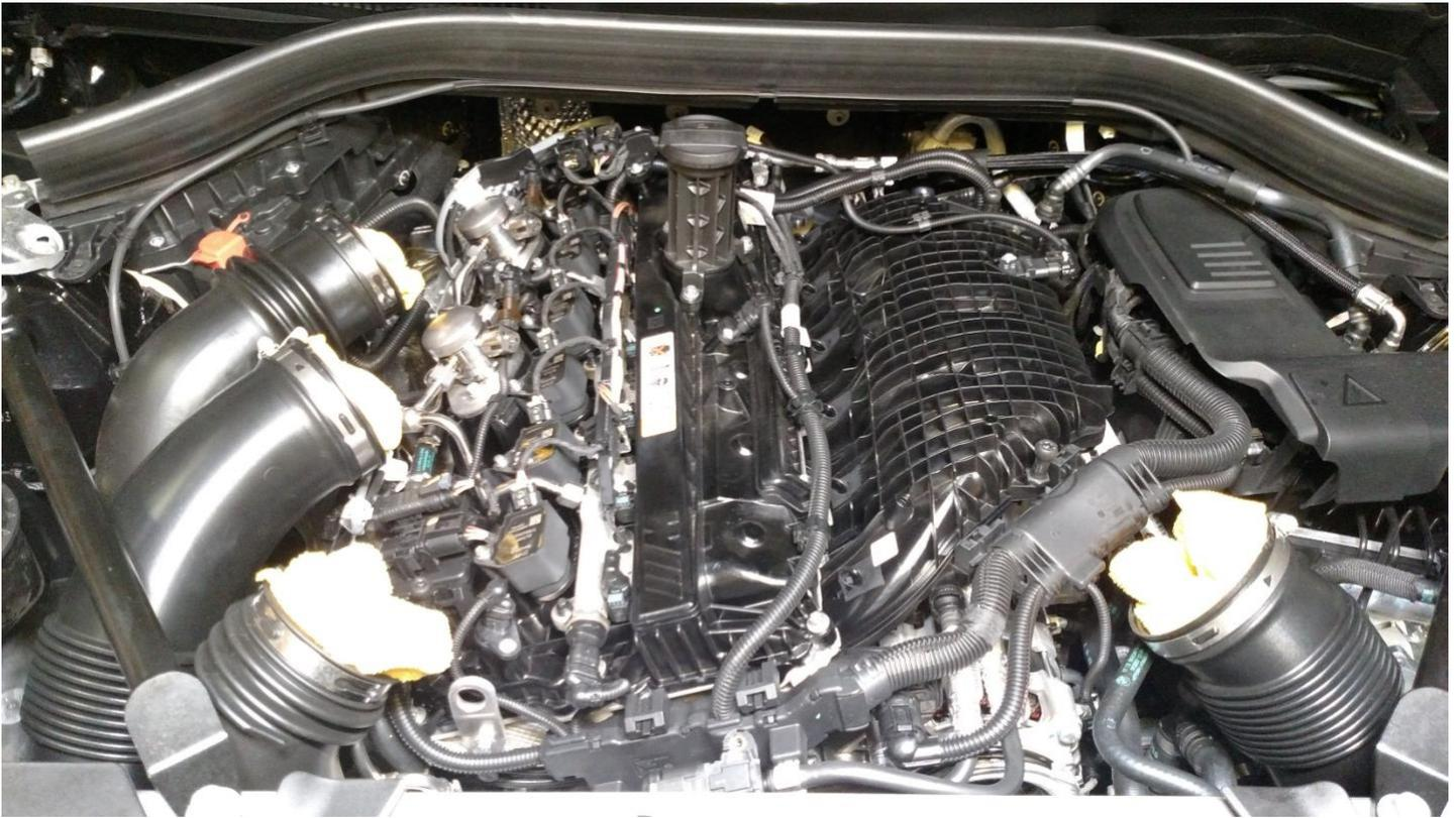
We suggest mounting/placing the JB4 on the driver side of the engine bay under the plastic cover. It can be zip tied to the strut brace or tucked out of the way. If equipped with the optional JB4 mobile adapter try to locate it so that it is not touching metal which may reduce its range. Also avoid mounting the box or wires too close to the wiper arm assembly which will move when wipers are turned on.
