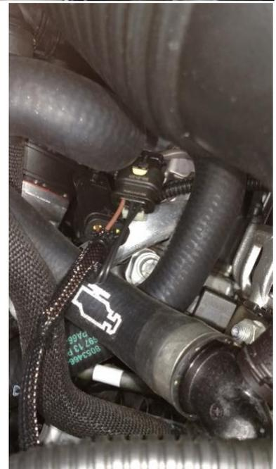
For the M3/M4 you can access the sensor from the top by removing the driver side airbox. Note the connection is down there so if you're able to reach it without removing any parts you're attaching it to the wrong spot. The AC condenser pressure sensor is nearby and often confused for the TMAP sensor.
