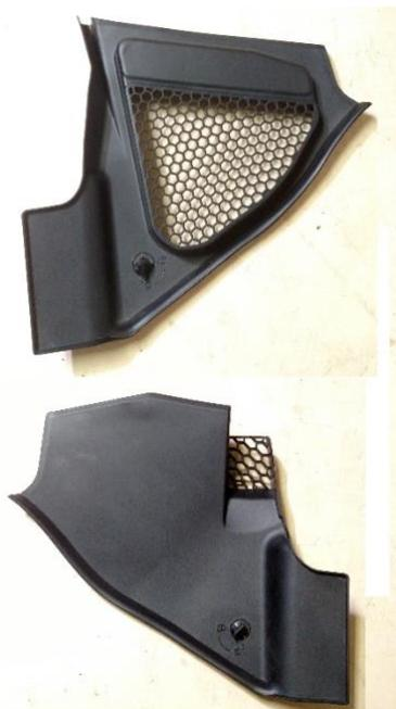
To remove the covers near the windshield, unlock as shown and lift the covers. Remove the pins around the strut brace and pull the rubber covers back to access the strut brace bolts.
