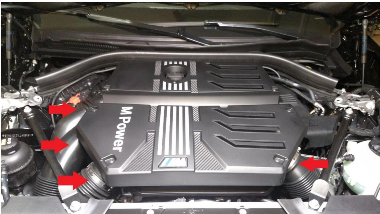
Remove the intake filter assembly by pulling straight up on the assembly and plug intake hoses with towels so that nothing can accidentally be dropped in to them.
