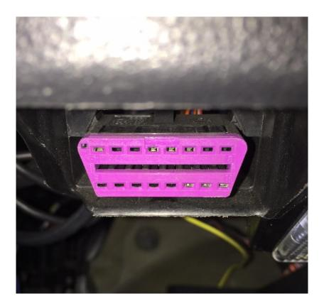
The OBD plug will go into the engine bay as per LHD instructions by passing over the centre tunnel just above the foot rest. Use a guide and tape the end of the OBD plug and start by passing it over the centre tunnel through the gap in the back. Pictured below is the wire taped to a long enough cable tie.
