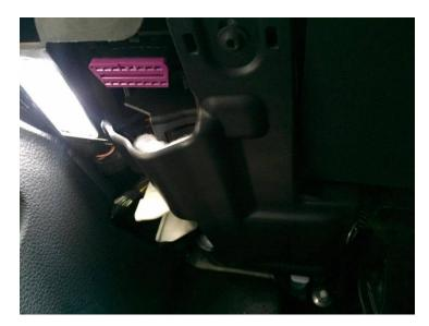
The panel can be removed by removing the hex screws holding it in place. Remove the insulation foam and this will expose a grommet that can be punched to get the wire pushed into the engine bay. In order to avoid removing the battery a wire guide or cable tie can be used by taping onto the end of the OBD wire.
