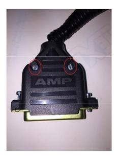
Once the cover is removed the wired pins can be pushed into the connector. The pins are numbered as below when viewing the pin side.
