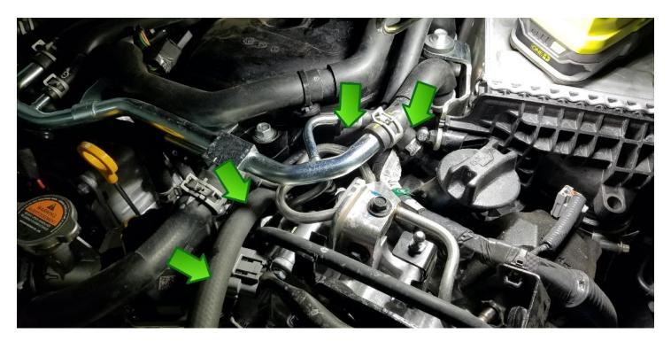
Next route the longer supplied 3/8" hose to the factory nipple on the intake manifold shown in the top of the photo below to the "OUT" nipple on the BMS oil catch can. Route this hose underneath the factory tubes in the vehicle to allow room for the engine cover to snap back into place.
