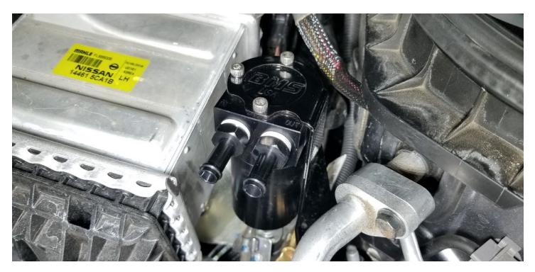
Remove the factory pressure clamp by squeezing it and sliding it back on the hose and pulling the hose off of the nipple with a flat head screwdriver or similar tool. We recommend leaving this hose in the vehicle as it's hard to remove/install.
