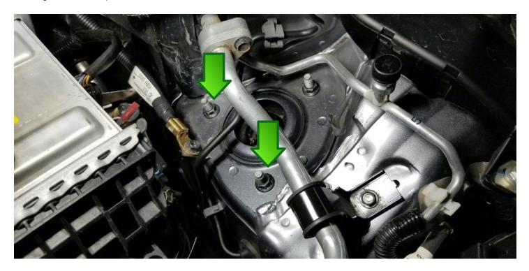
Next place the included bracket pictured below on the studs on the shock tower and replace and tighten the bracket down with 12mm shock tower bolts that were just removed.
