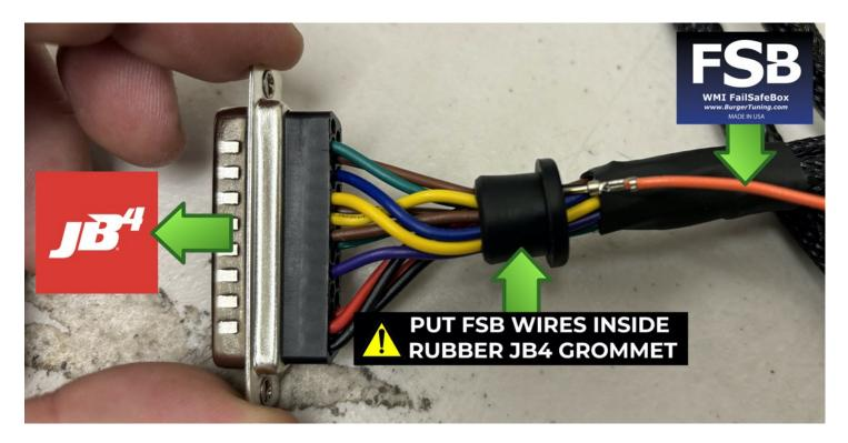
Pay special attention to this step. The pin holes in the DB25 connector are numbered.
