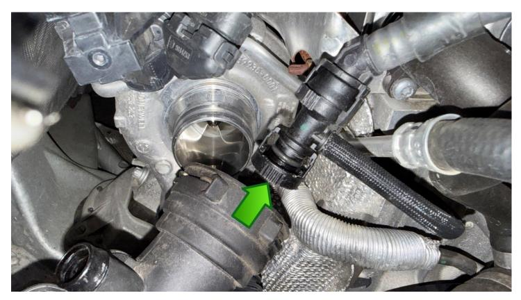
Click the inlet on to the turbo and be sure it's securely clipped on before proceeding. Next clip the rear breather hose on to the smaller fitting. Next click the PCV hose into the larger fitting.
