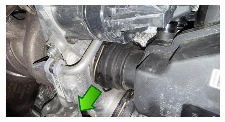
Carefully remove the PCV hose from the factory inlet by simultaneously pressing in the clips in on each side and pulling upward.
