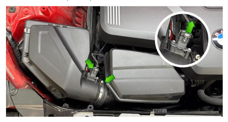
Prepare by adding the supplied black silicone O-ring and metal clip as shown below. A little lubricant/oil on the O-ring will help the inlet go on easier during the install.
