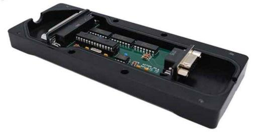
2) Install the DB9 connector and ensure both screws are secure.
