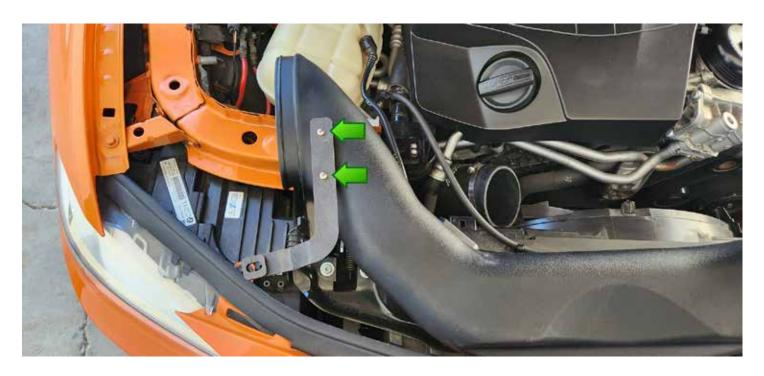
7. Carefully Place the air filter on the intake tube. The filter pleats will distort if too much force is used. Hand tighten the filter clamp with a screwdriver until the filter is secure. Do not over tighten or the polymer tube will distort and cause air leaks.
