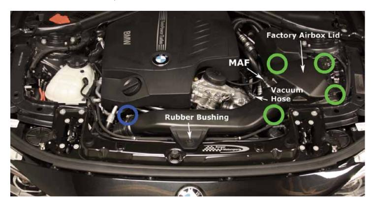
3. Remove the MAF sensor by unscrewing the (2) T20 Torx screws. Screw those back into the factory intake for safe keeping as they will not be reused with the BMS intake.
