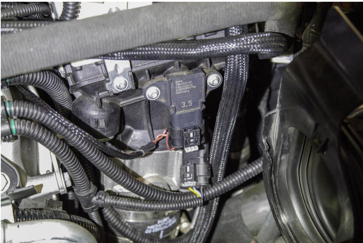
On the driver's side, find the TMAP sensor. Note that the factory connector on this side is a different style. It does not have a locking mechanism and is removed by pressing on the small squared off section shown in the below photo. Press at this section and remove the factory connector.
