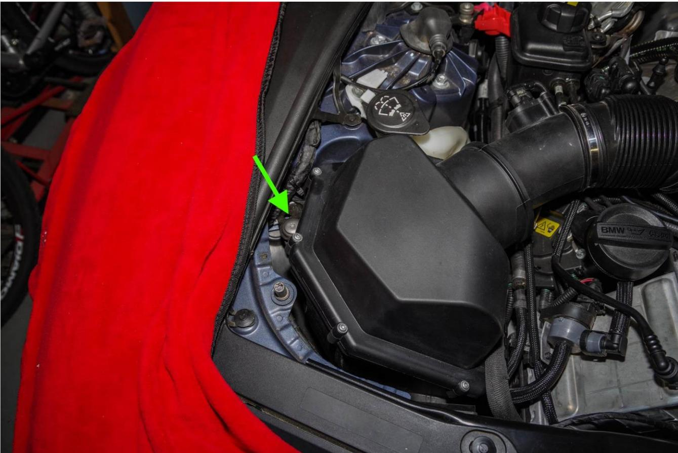
Now loosen the clamp nearest the turbocharger inlet housing using a 6mm socket and ratchet or a screwdriver. Loosen the intake hose from the housing that connects it to the front of the turbocharger, where you loosened the clamp, by pulling the accordion section back from the housing.
