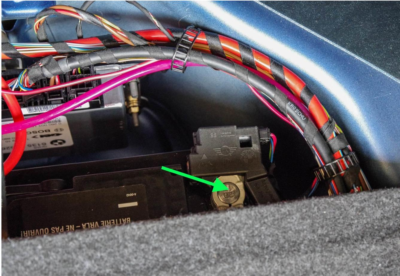
**The battery is now disconnected. Do not close the trunk until after you have reconnected the battery or you will not be able to reopen it.**
