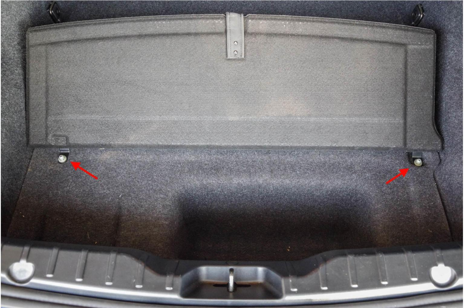
Remove these nuts and set aside, raise the trunk floor panel, and loosen and detach the negative terminal on the battery, now partially exposed, using a 10mm socket and ratchet.
