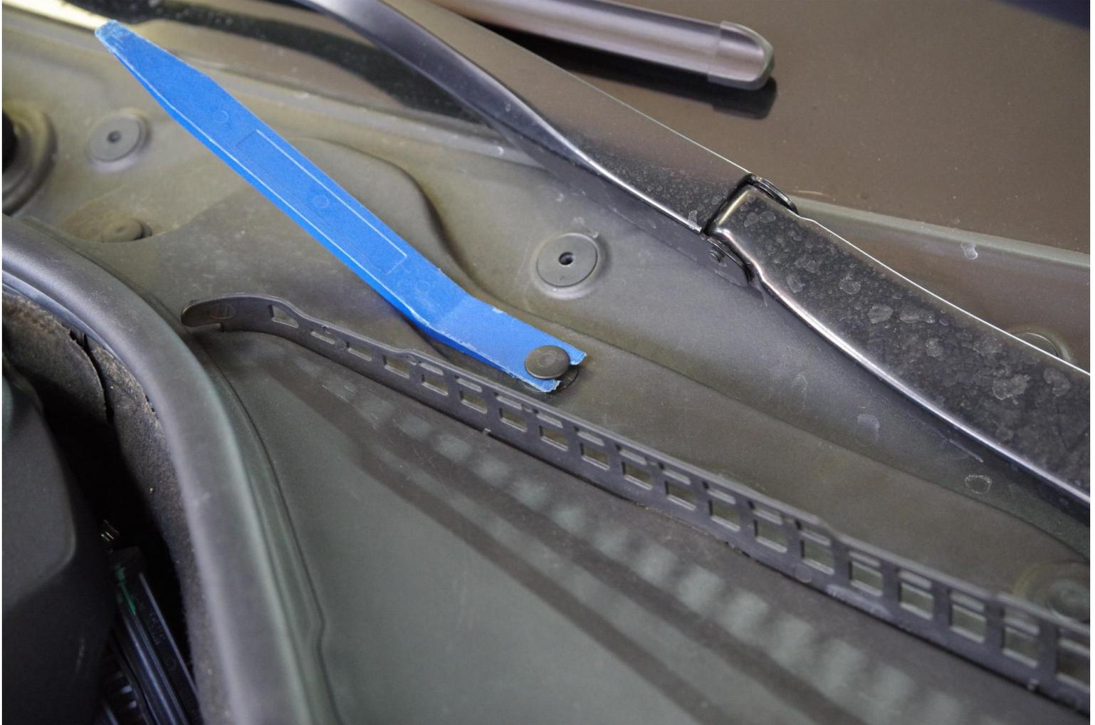
Pull up on the plastic cover to release it. Then pull the rubber hood seal away from the plastic to allow room to pass the control box and harness through to the corner compartment from the engine compartment, near the shock tower. A rubber cover allows clearance to pass the harness through.
