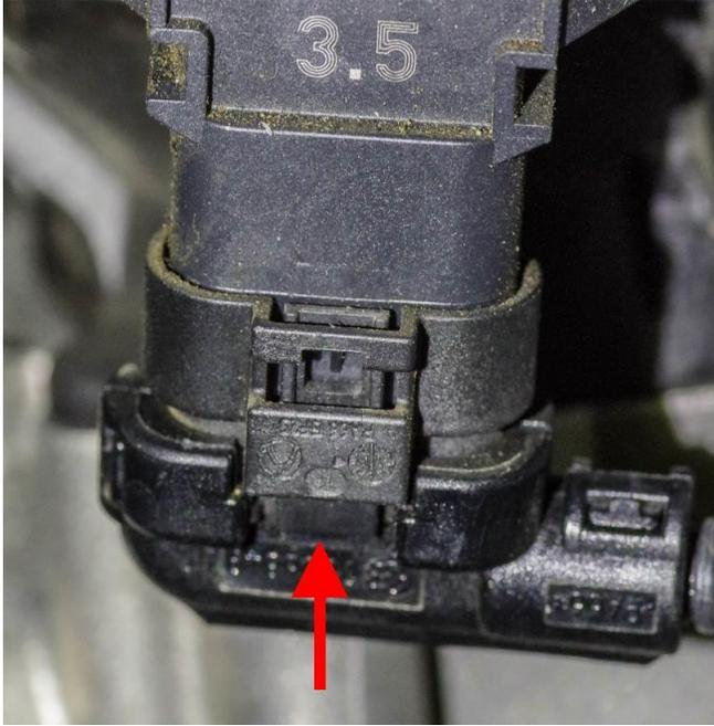
Now attach the tuner's rainbow female connector at the sensor and attach the factory connector you removed to the tuner's rainbow male connector, as shown.
