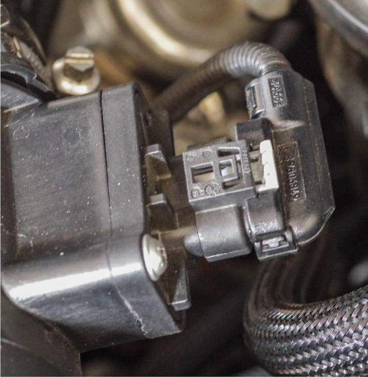
Do not pull from the wires. If the clip fails to release, you can apply slight pressure with a pry tool, or insert a small screwdriver to try to raise the retention tab as needed. Repeat for both MAF sensors (one on each intake). Remove the T30 Torx fastener shown in the attached photo.
