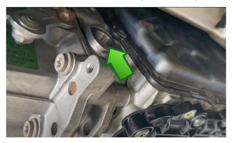
Now remove the fill plug on the side of the transmission again and top the fluid off until the fluid starts coming out again. Tighten to 18.4 ft-lbs (25 Nm).
