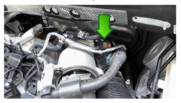
Line up the holes on the BMS BOV adapter with the holes on the factory bypass solenoid.
