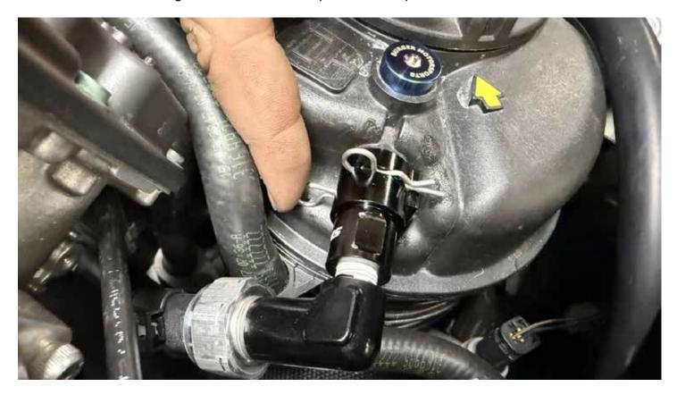
Install the connector to the sensor and route the wiring over to the JB4 system.
