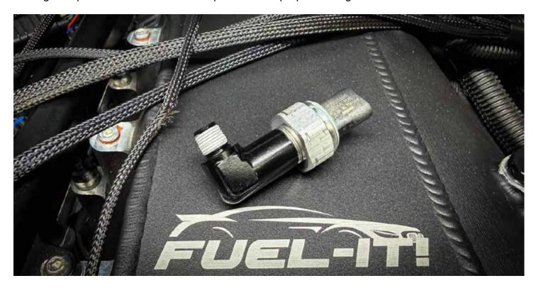
Lube the fitting on the tank to aid in installation.
