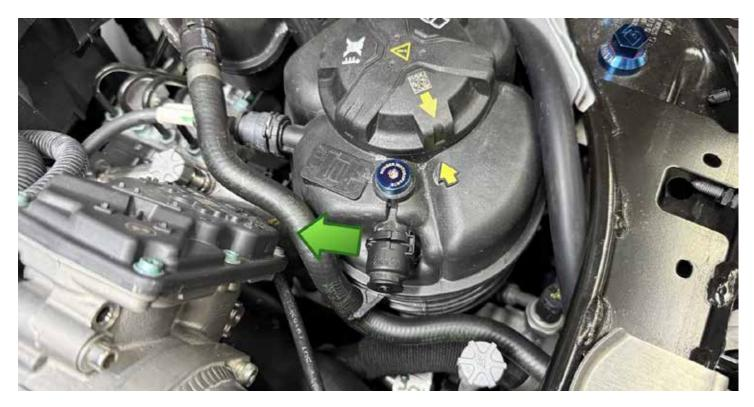
Place a rag underneath the fitting to catch any coolant.
