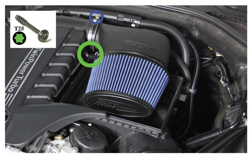
6. Place the intake outlet into the inlet hole on the car. Use the torx bolt you removed to attach the black bracket to the bottom half of the factory air box. This bolt is circled in green. Tighten the hose clamp around the BMS intake outlet. This bolt is circled in blue in the above photo.
