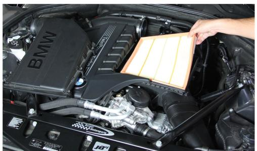
3. Remove the restrictive flat paper factory air filter. Set both the air box lid and the factory air filter aside in a safe place. 1 screw from the air box lid will be used to attach the BMS intake to the bottom of the factory air box with the supplied black bracket.
