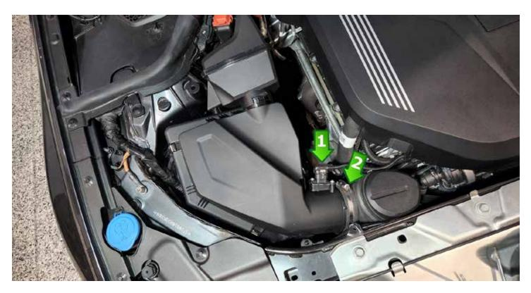
Remove the factory intake by pulling up on it. Be sure the 3 rubber supports are still in place. They may become dislodged during the removal of the factory intake.
