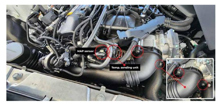
Unplug this cable by pinching the clips on the top and bottom and pulling outward.
