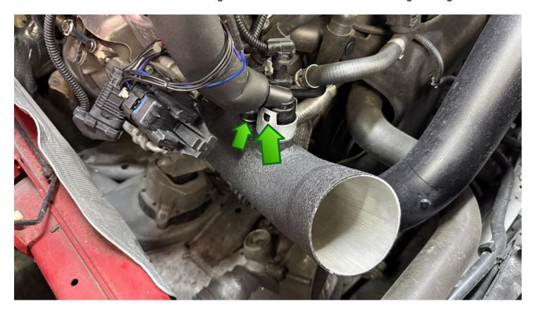
Now attach the silicone coupler and hose clamps to the B48 competition intake outlet.
