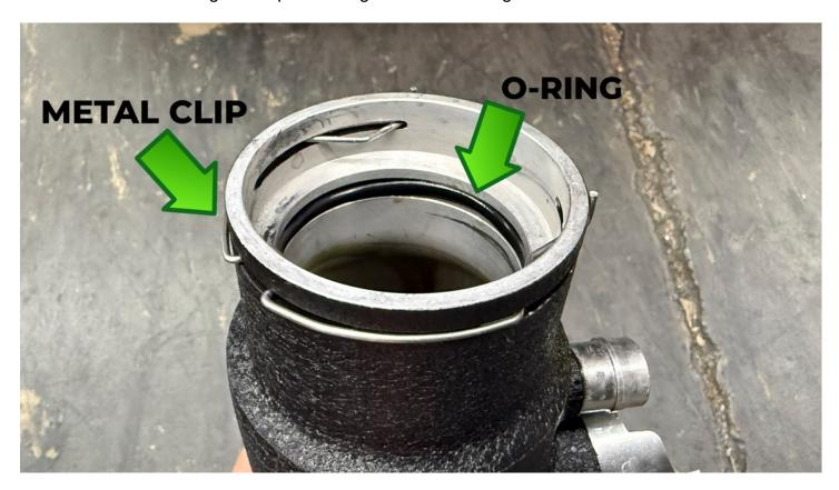
Next pull the metal clip out from the factory inlet turbocharger connection and pull the tube off.
