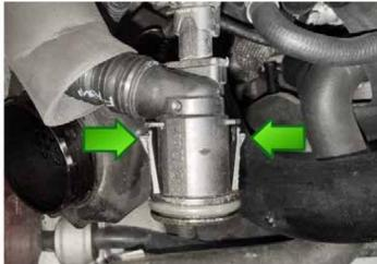
Now remove the other breather hose from behind by pinching the front at back on the vertical lines (IIII) and pulling upward to release.
