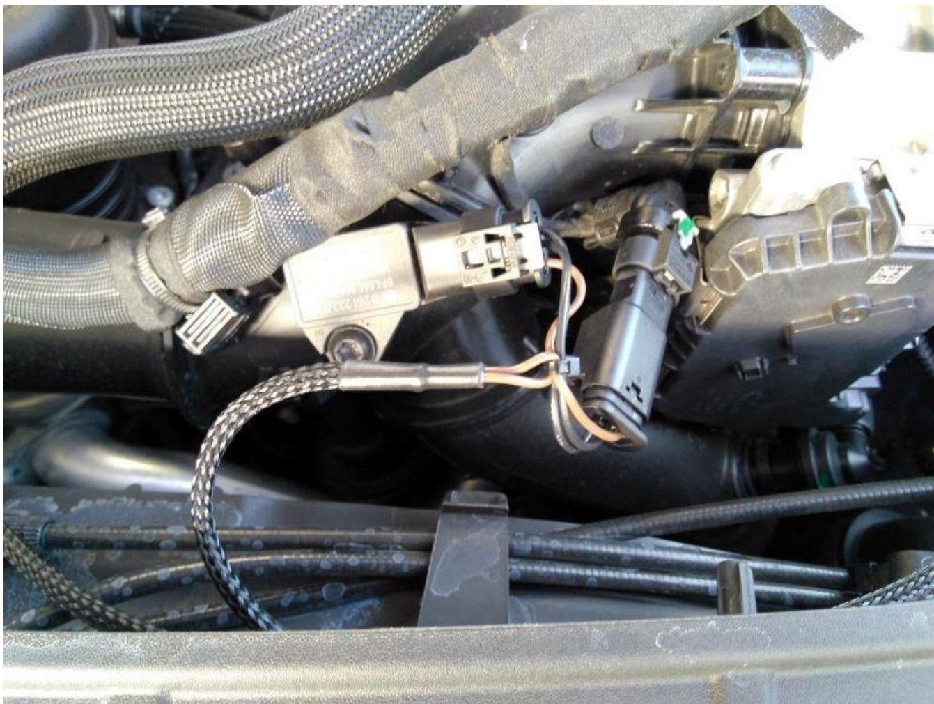
**Fuel Pressure:** Green/black patch on JB4 harness. This connection is optional and the connector on the fuel pressure sensor can be tricky to release. During development we found the easiest way was to use a longer screwdriver to apply pressure to the base of the connector while pressing the clip in. This connection will come in to play if you plan to mix in E85 fuels. If not planning to use E85 you can skip it at least initially.
