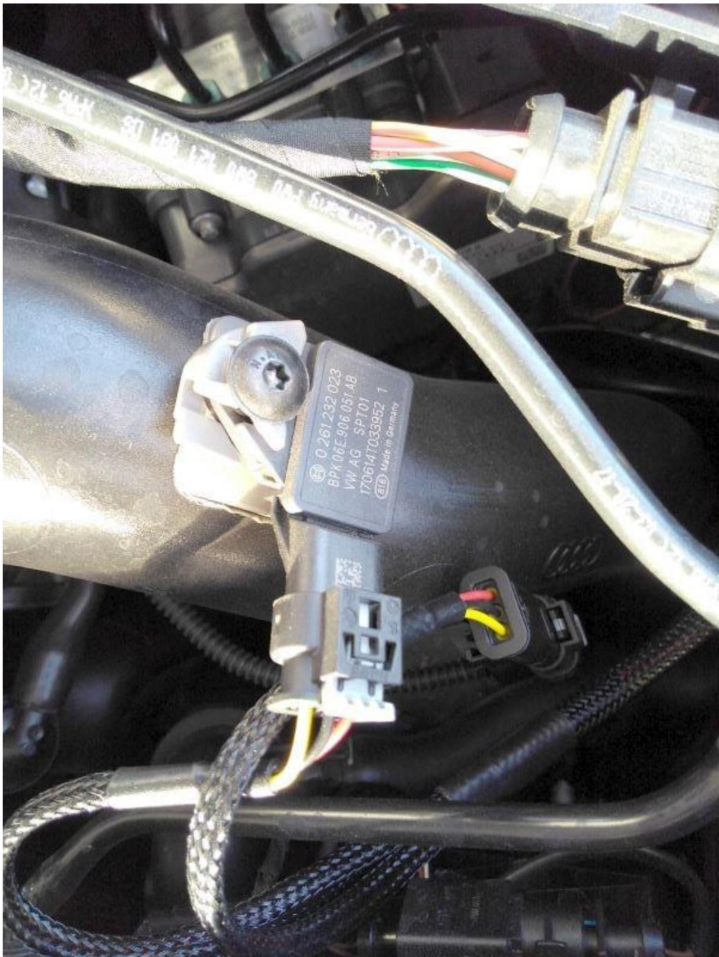
**MAP: Brown patch on JB4 harness. Unplug the factory connection, plug the JB4 harness in to the sensor, and plug the factory connection in to the JB4 connector, completing the loop.**
