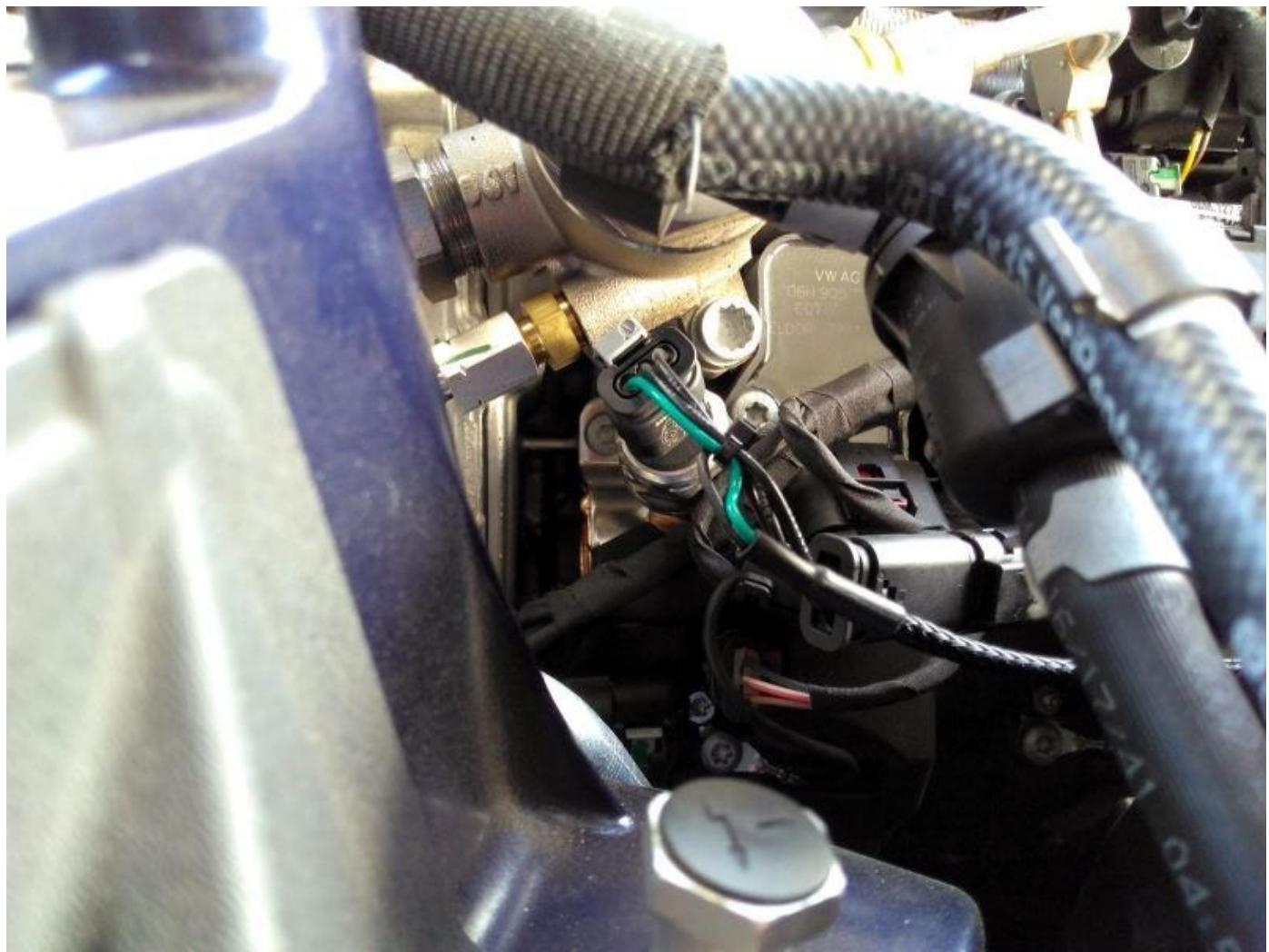
**OPTIONAL BCM Connector (boost control module) standard on Revision 2 units:**
