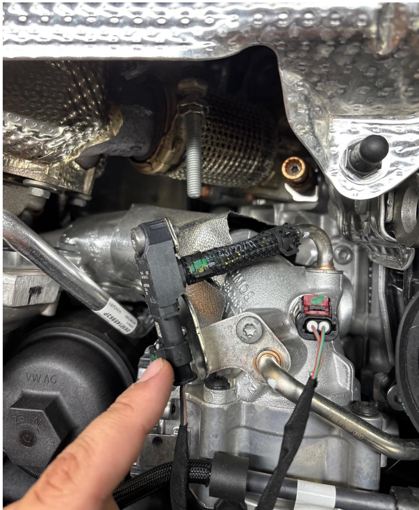
To access the passenger side boost sensor, you may need to partially remove the air inlet tube.
