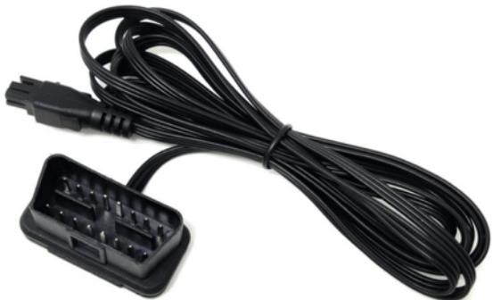
The easiest way to route to the engine bay is around the doorjamb. Alternatively, it can be run through the firewall behind the pedal assemblies via existing grommets. Finally plug OBDII into JB4 harness, noting correct clip over notch orientation. If no data appears in the JB4 app once connected an issue with the OBDII connection is usually the culprit.
